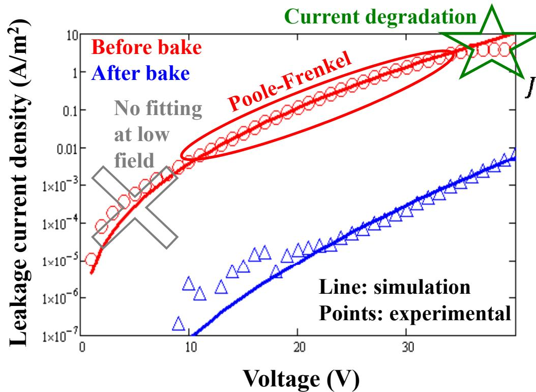
$$J_{PF} = A_{PF} \times \frac{V}{t_{ox}} \times e^{-\left(\frac{q \times \Phi t}{k \times T}\right)} \times e^{\left(\beta_{PF} \times \sqrt{\frac{V}{t_{ox}}}\right)}$$
