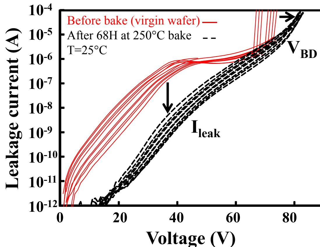
➤ Bake impact →  $I_{leak}$  decreases and  $V_{BD}$  increases
